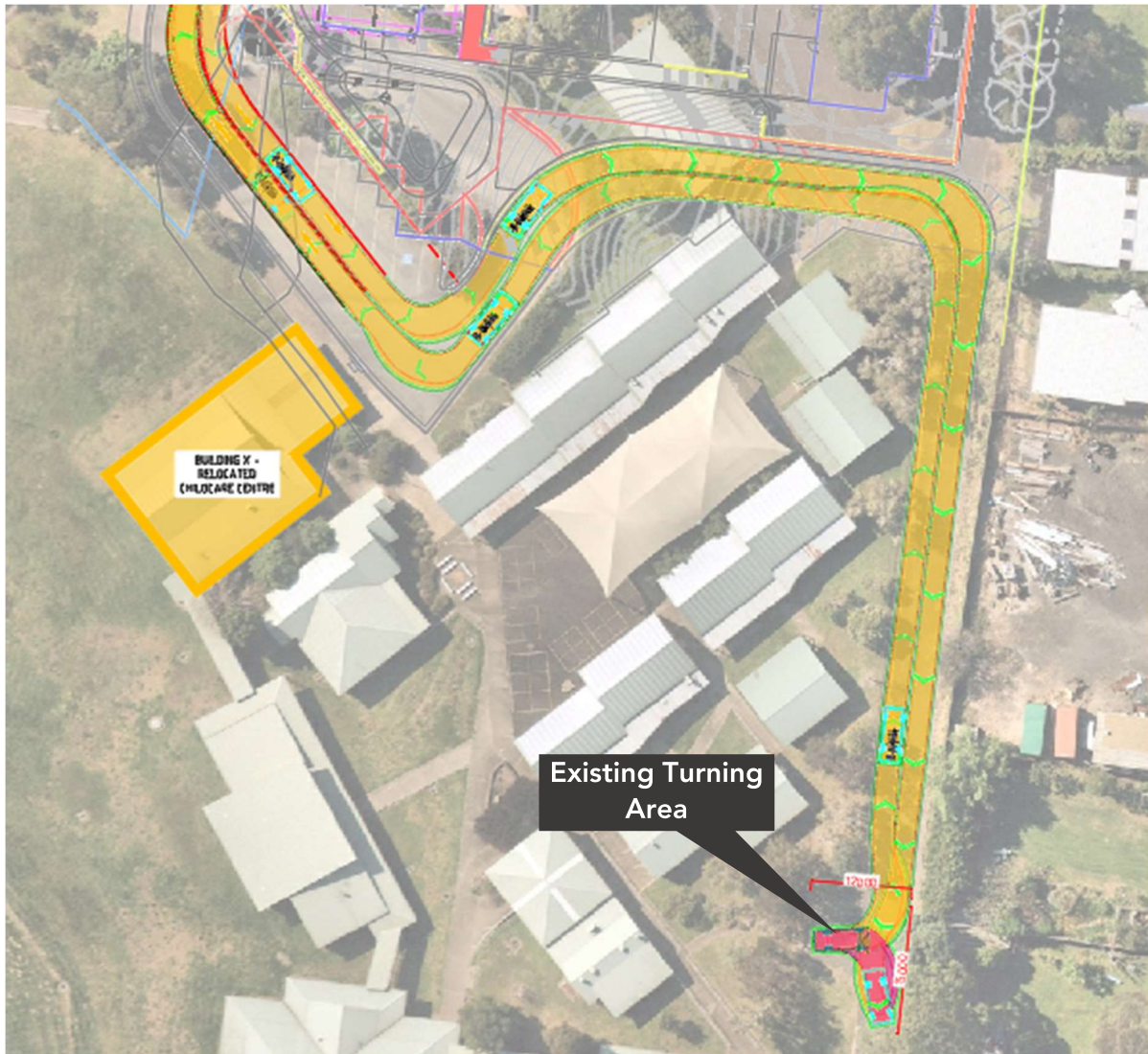
Figure 3 - Existing Turning Area with 6.4m SRV Swept Path
